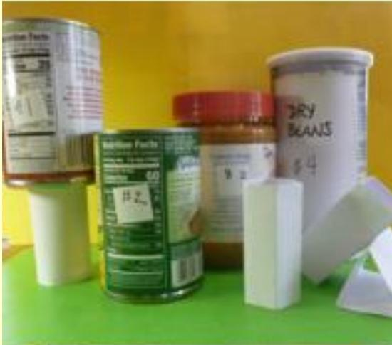
For Steps 4-6: Assemble a series of weights, numbered 1, 2, 3 and 4, then test all four tubes with #1; then all four with # 2, then #3, and #4, writing down which tubes hold up the weight without collapsing each time.
