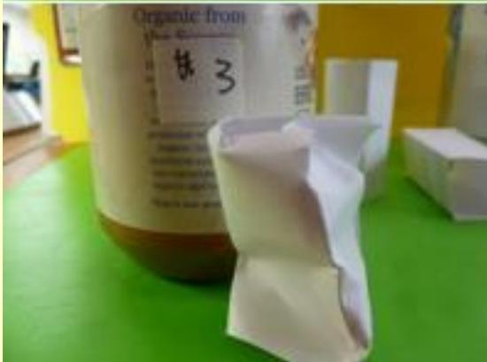
For Step 6: Oops! My poor little triangle tube **collapsed** with Weight #3----good thing I had my hand right on that plastic jar so I could catch it before it fell down!! I marked Triangle – #3 – “**No**” on my table of results.
